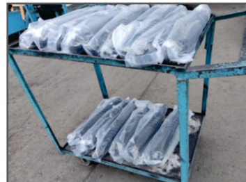
No proper arrangement for keeping the damper during dispatch
