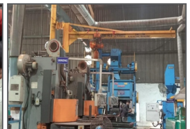
Grinding plate loading through Jib crane
