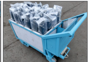
Now we have made a trolley for keeping the damper during dispatch
